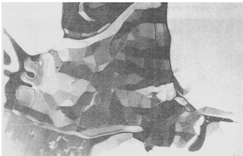
FIGURE 8 A lot of subgrains, appearing in a pseudoisotropic grain after deformation.
