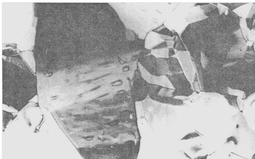
FIGURE 5 Long axes of dimples are parallel to n_y in the three regions of a large grain.
